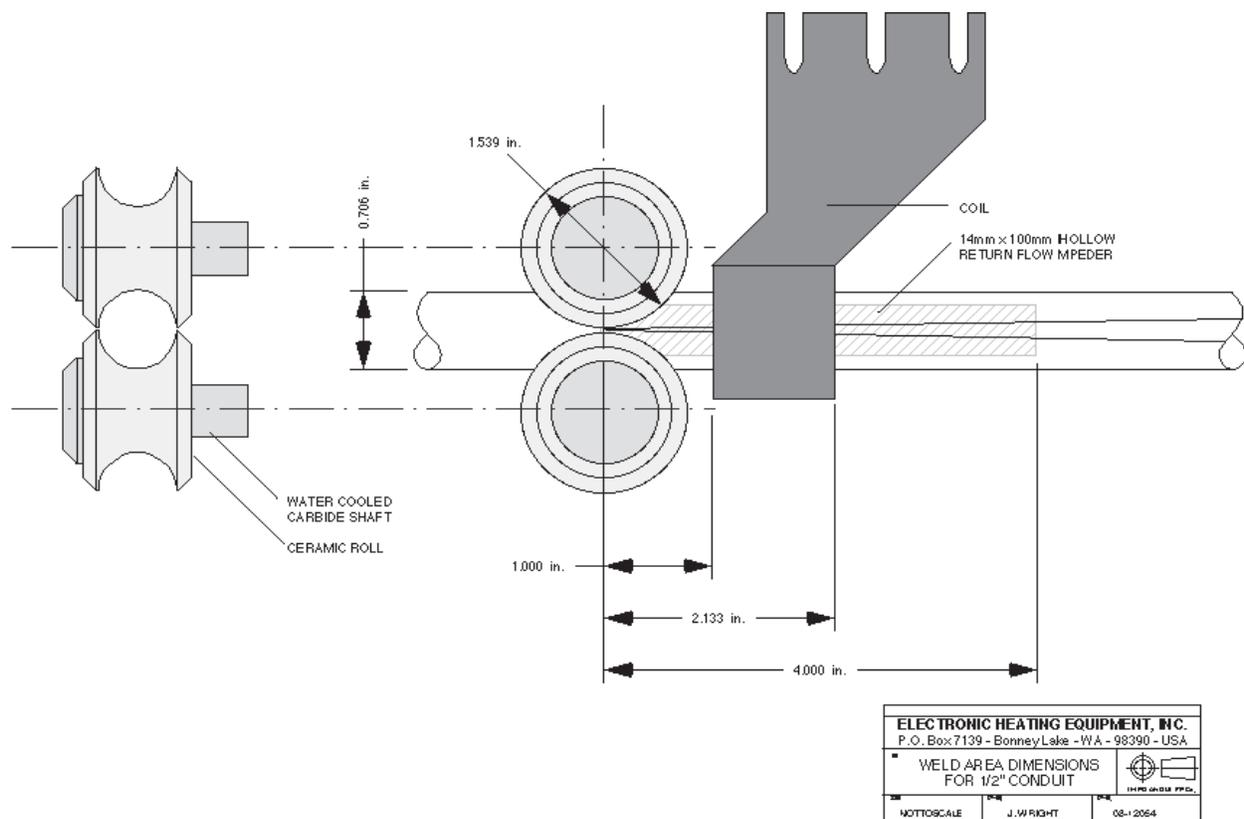
Welding 1/2" and 3/4" EMT conduit at speeds of 1000 ft. per minute does not require a lot of weld power. With an efficient setup, 250-300kW should be adequate.
