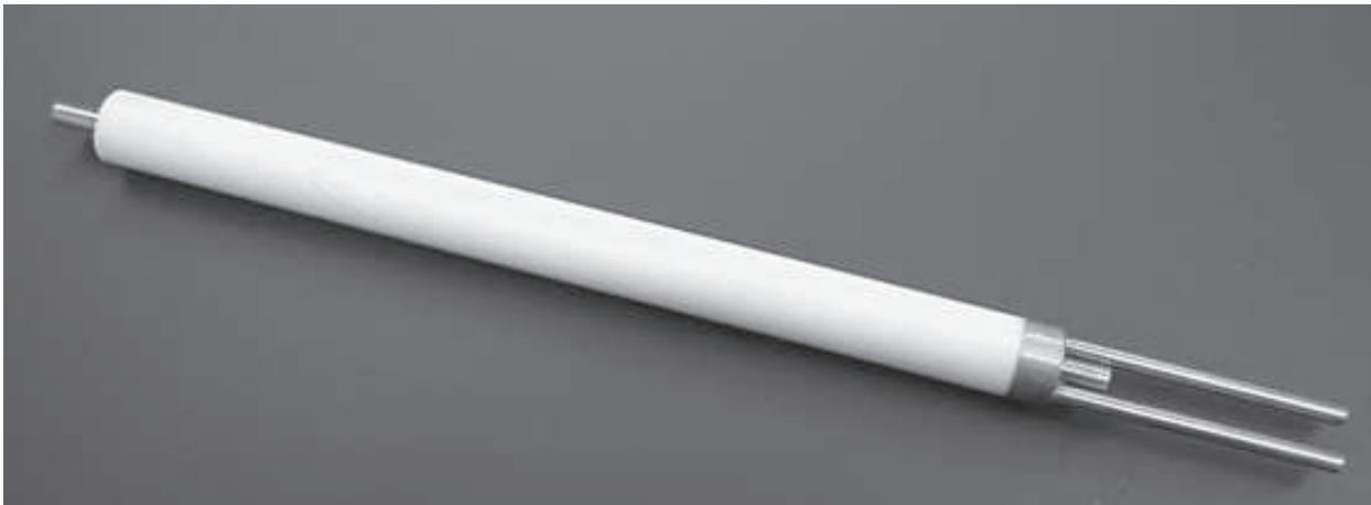
A typical impeder for welding 1/2" EMT conduit is 14-15mm in diameter & 230mm (9") long. It has a 4-5mm (5/32" - 3/16") hole through the center for the paint & nitrogen, and two 3mm (1/8") coolant lines. The ferrite generally consists of a bundle of small diameter cylindrical rods. The outer case of the impeder is usually high temperature resin bonded glass fibre tube.
